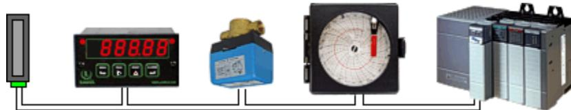
**Not so good:** A single 4-20 mA loop from a sensor is connected to a panel meter, a control valve, a recorder and a PLC in series. If the loop opens, all devices in the loop fail.
