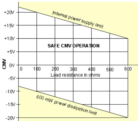
**Common mode voltage:** If a load R is grounded to a Remote Ground, the available common mode voltage CMV is limited on the positive side by the unit's internal power supply and on the negative side by the 600 mW power dissipation limit of an output transistor.
